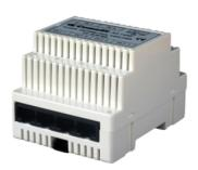
Floor distributor (switch) for IP door entry monitors for routing the data packets of the Comelit ViP system. Equipped with 6 Ethernet communication ports with Comelit PoE (10/100Mbit/s). Product 1440A negotiates the connection speed depending on the connected devices, and the Comelit PoE allows cascade power to be supplied to several 1440A products by enabling the system to be connected over longer distances than the PoE standard. Dimensions: 71x89x62 mm (4 DIN modules).
